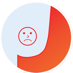
incorrect chamfer preparation
