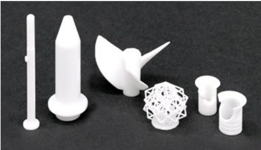
Various geometries produced with ceramic 3D-printing
